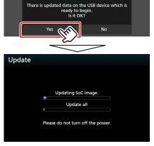
**Caution:** The screen may go blank for a few seconds. Do not unplug the USB memory or Power Off the unit during the Update Procedure.
