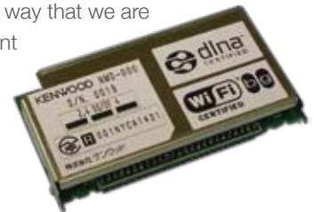
NMD-000 small data communication module incorporating the 2007 DLNA guidelines
