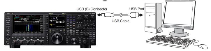
The KENWOOD TS-990S is equipped with a USB (B) connector for exchanging both of audio signals and PC control commands for performing data communication with an external device such as a PC.
